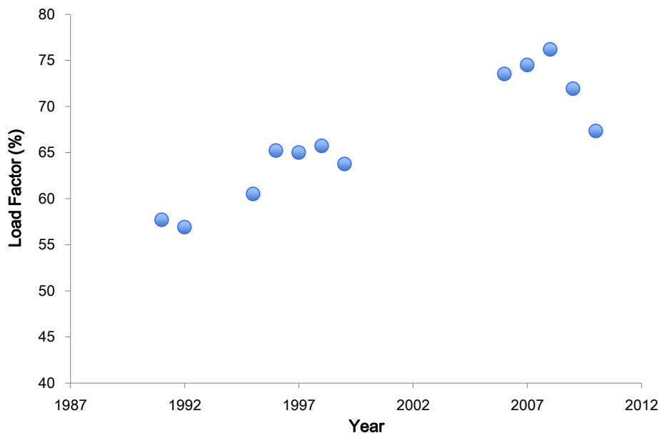
Figure 8. Load Factor: The load factor is a fraction representing how much generation capacity is required in a system versus how much electricity is consumed on average. From a utility's perspective a higher load factor is better since revenues are roughly proportional to average production but fixed costs are proportional to maximum demand ( Source: Duncan Callaway. Electric Power Systems 254 Class Notes, UC Berkeley ). In a constant pursuit to increase load factor Gujarat's utilities were benefited by the Yjotigram scheme which usually provides overnight three-phase power to farmers on a pre-arranged schedule ( Data Source: India's Central Electricity Authority ).
